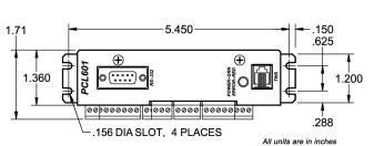
PCL601 Programmable Controller provides you with a complete motion solution in a compact package. It simplifies programming tasks and provides the essential features for any positioning system. Say goodbye to PLC's and time consuming Ladder Logic Programs for good. The PCL601 features the ability to connect to a PC and instantly provide movement for a stepper motor. Whether you require a stored program, or the ability to send serial text instructions, this versatile controller.
